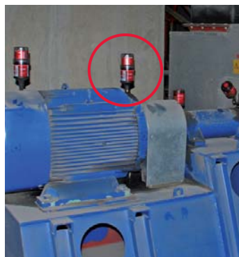
Drive motor lubrication (2 points)
