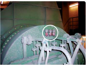
(above left) **Bearings** Bearings are effectively sealed against aggressive cement dust and other contaminating substances.
